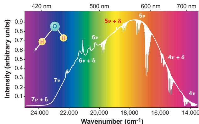
**Now you see it.** The visible absorption spectrum of water, recorded with a high-resolution Fourier transform spectrometer and a long-path absorption cell. The overtones are the small modulations of the spectrum. (**Inset**) The water overtone O-H stretch. [Adapted from (15)]
