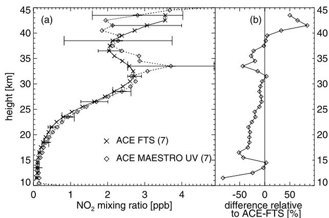
**Figure 5.** (a) Mean NO<sub>2</sub> profiles measured by ACE-FTS and the ACE-MAESTRO UV spectrophotometer using seven profiles to calculate the means, and (b) the mean of the differences relative to the ACE-FTS profile:  $(ACE-FTS - x)/ACE-FTS$ .
