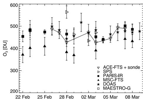
**Figure 2.** O<sub>3</sub> total columns measured by the three UV/visible spectrometers and the two ground-based FTSSs, and the derived ACE-FTS total column. The line shows the ACE-FTS variation.
