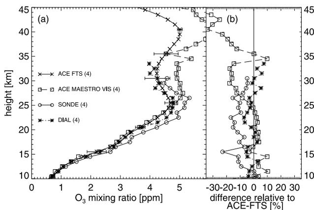
**Figure 3.** (a) Mean O<sub>3</sub> profiles measured by ACE-FTS, the ACE-MAESTRO visible spectrophotometer, ozonesondes and the DIAL, using four profiles to calculate the mean, and (b) the mean of the differences relative to the ACE-FTS profile:  $(ACE-FTS - x)/ACE-FTS$ .
