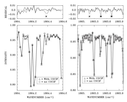
Fig. 2. Bottom panels: comparison of averages of all ACE tropical spectra measurements in 2004 at latitudes between 20°S and 20°N and altitudes between 22 and 24 km obtained with the best-fit COCIF profile with those obtained assuming the COCIF mixing ratio is zero at all altitudes. Upper panels: residuals (measured minus calculated signals) on an expanded vertical scale. Asterisks mark locations of stronger COCIF features in the sample intervals.
