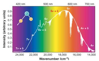
**Now you see it.** The visible absorption spectrum of water, recorded with a high-resolution Fourier transform spectrometer and a long-path absorption cell. The overtones are the small modulations of the spectrum. (Inset) The water overtone O–H stretch. [Adapted from (15)]
