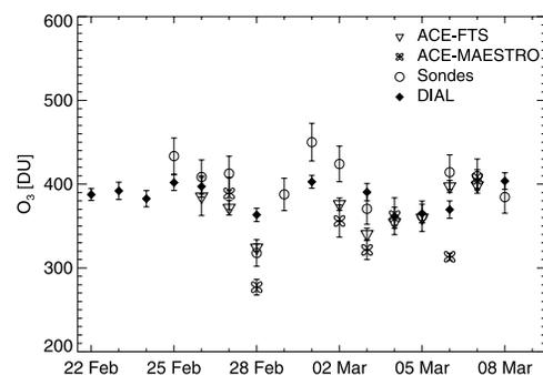
**Figure 1.** O<sub>3</sub> partial columns (10–30 km) measured by ACE-FTS, ACE-MAESTRO, the DIAL and the ozonesondes.
